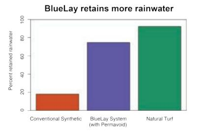
With 80% open volume, BlueLay will store 24mm (1 in) of water. When fully wetted, the natural capillary action of stone wool can provide an average of 6-8 days cooling performance without any rain! Add a sub-base of Permavoid for an additional 75mm (3 in) of water storage and cool your field even in the hottest, driest climate.
