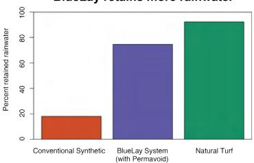
With 80% open volume, BlueLay will store 24mm (1 in) of water. When fully wetted, the natural capillary action of stone wool can provide an average of 6-8 days cooling performance without any rain! Add a sub-base of Permavoid for an additional 75mm (3 in) of water storage and cool your field even in the hottest, driest climate.
