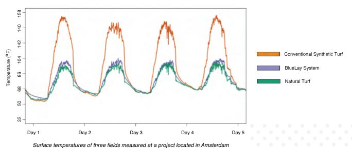
BlueLay is more than just a shock pad. It is a water retention and drainage layer designed for use directly below synthetic turf. Its revolutionary design provides sport technical performance, stormwater management functions and, most importantly, synthetic turf cooling.
