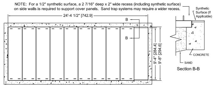
NOTE: Typical sand pit requiring 10 cover panels shown, one cover is removed. For longer sand pits, add 29 1/4" for each additional; panel required.
