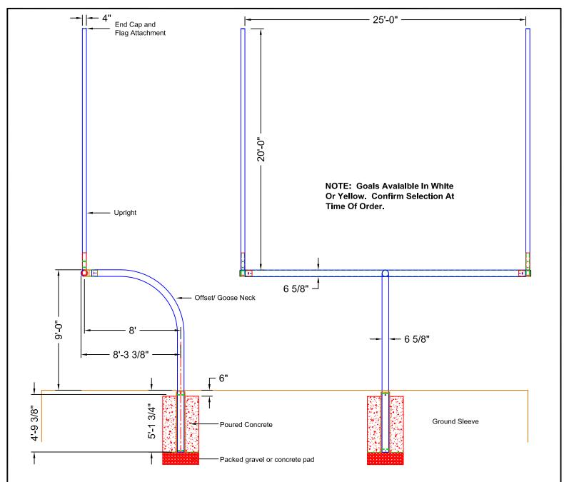
NOTE: Contractor / Installer shall consult codes and soil condition for final foundation depth and size.
