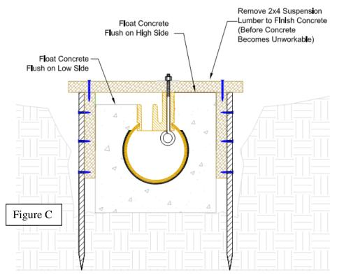
9. Pour concrete encasement being careful not to chute concrete directly against the XT-8 Collector. Concrete should be brought up to the top of the form on the track side and <u>only up to</u> <u>the level of the drain slots on the</u> <u>field side</u> (Figure C). Be careful not to move the channels out of alignment during concrete placement. Distribute concrete evenly. Use a rod to completely consolidate the concrete during concrete placement.
