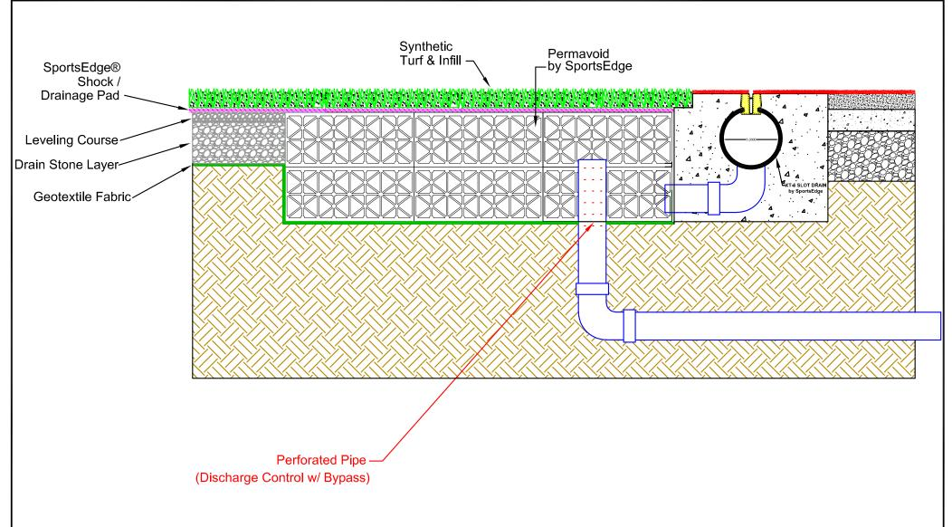
Plan View- SportsEdge XT-6 Surface Drain System w/ Shock/Drain Pad and Permavoid Water Control System
