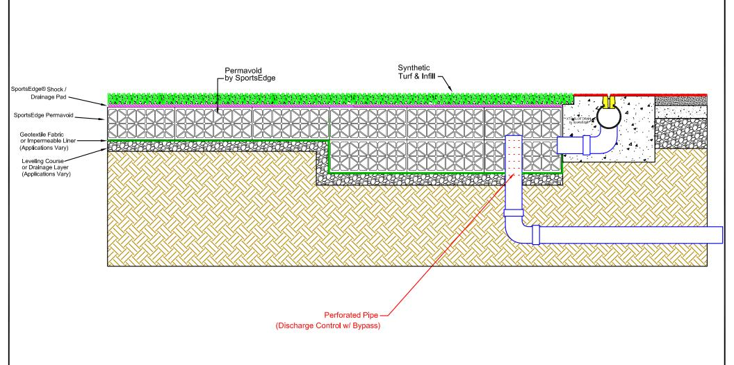
Plan View- SportsEdge XT-4 Surface Drain System w/ Permavoid Raft / Water Control System
